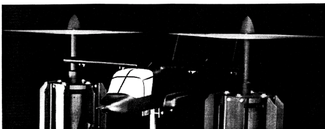
Fig. 1 Eight percent model of the XV-15 tiltrotor in hover.
